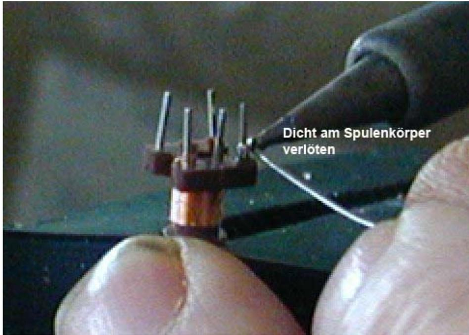
under the direct control of your eyes and you can lay one turn next to the other without difficulties. Do not forget to count the turns :-)
