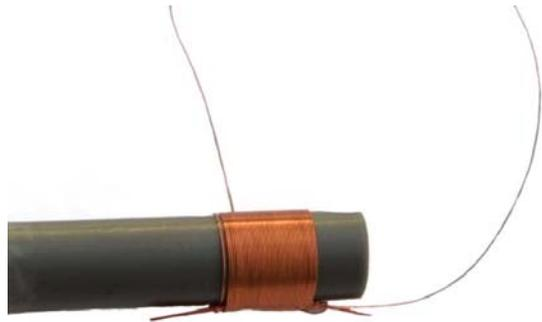
**Here you see the ready wound VFO coil. Solder the ends of the wire after installation to their solderpoints at the PCB.**
