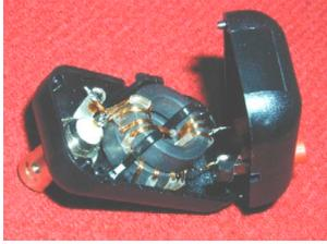
If you want to use the balun in the QRPproject format, prepare the enclosure and solder the UNBAL part as short as possible to the BNC connector. The BAL side has to be soldered to the two 2mm banana jacks.
