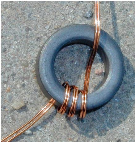
The 4th turn goes through the toroid and ends at the opposite part of the toroid as shown in the picture above.
