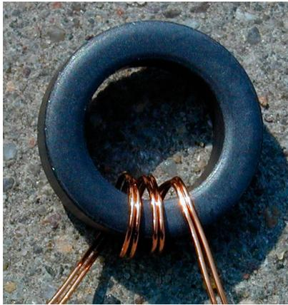
Count the turns INSIDE the toroid. The picture shows 3 turns.
