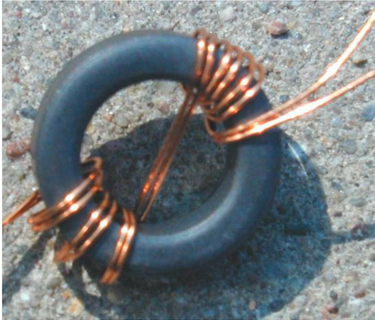
At the opposite again count 3 turns. The complete count now is up to 7 turns. The reason to cross the toroid is to have start and end of the turns at opposite ends of the toroid. At both sides of the toroid you should have a short and a long end of wire now.
